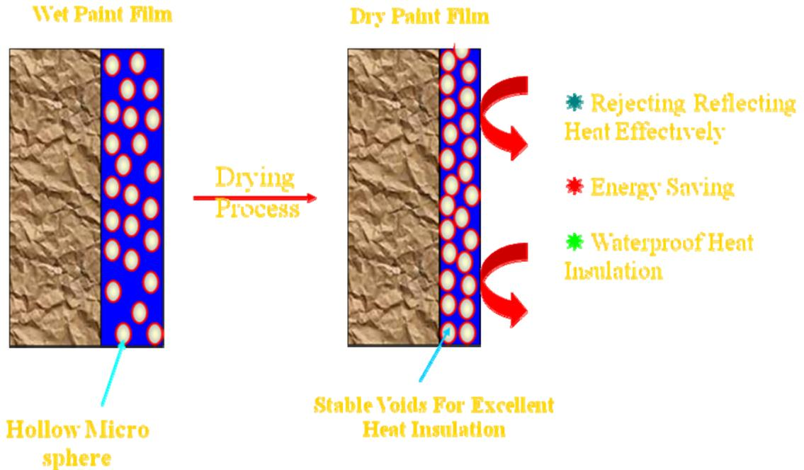
Figure 1. Mechanism of heat insulation of exterior heatshield coating
