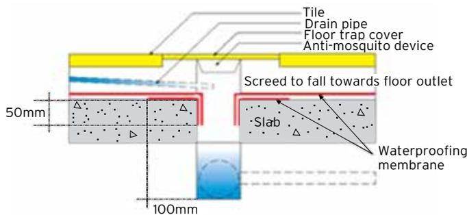
Fig. 15: Waterproofing details at floor outlet
