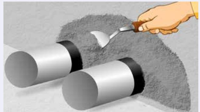
Fig. 22: Fixing the pipes with sealing tape and further doing the grouting
