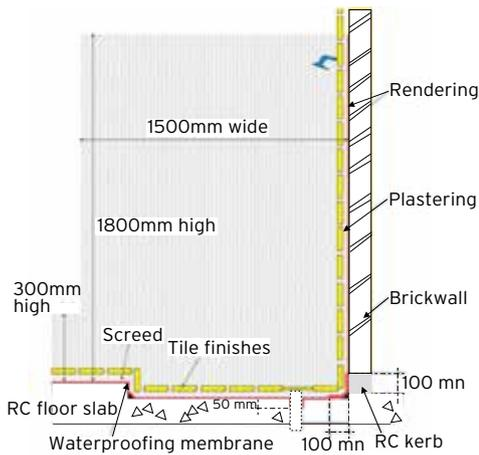
Fig. 9: Waterproofing details of shower area
