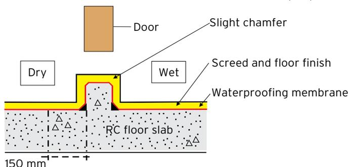
**Fig. 6:** Kerb between wet and dry area
