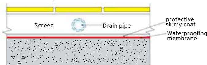
Fig. 16: Pipes embedded in screed
