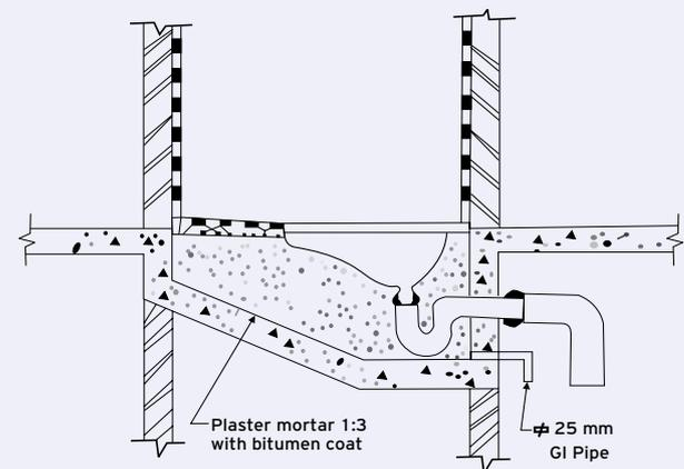
Fig. 2: Depressed slab and arrangement of joints in WC
