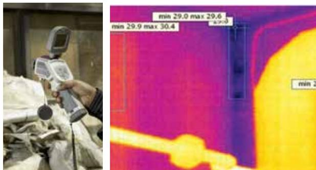
IR Thermography to detect delamination and voids of concret as well to find out the source of water leakage and location of water pipe
