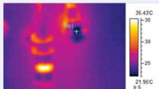
**Fig. 8:** Source of water leakage (+) being identified by thermal imaging
