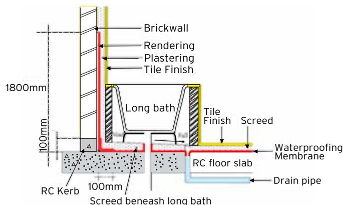
Fig. 11: Detailed cross section at long bath area
