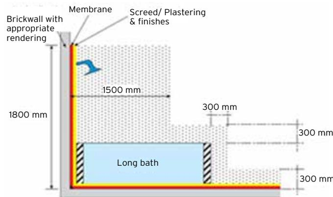
Fig. 10: Waterproofing details at long bath area
