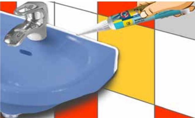
Fig. 31: Filling the gap with acrylic sealant
