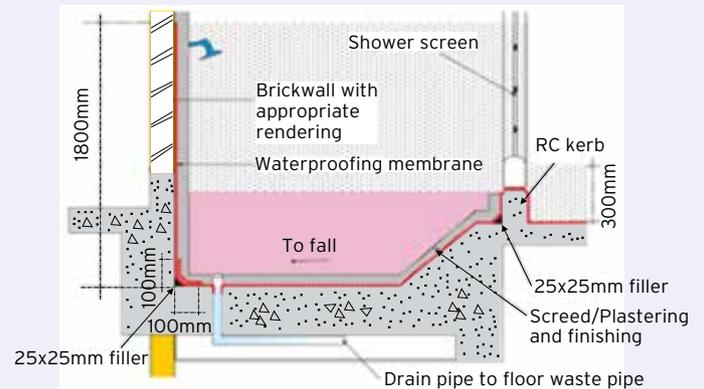
Fig. 12: Waterproofing details at sunken bath
