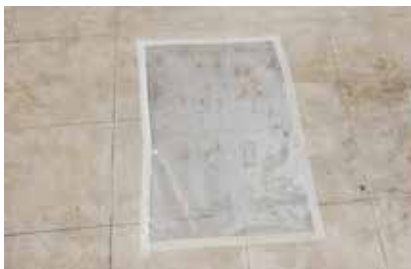
Fig. 16c: Checking the moisture content of the substrate by enclosing with polythene sheet
