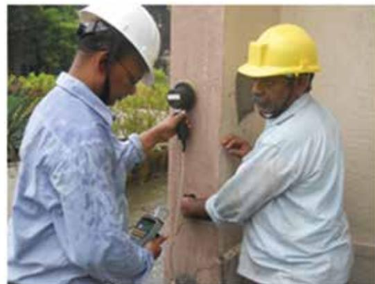
Measuring the rate of corrosion in steel reinforcement by Galvanostatic Pulse measurement
