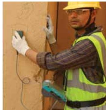
Measuring the cover depth with a Profometer
