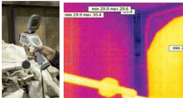
IR Thermography to detect delamination and voids of concret as well to find out the source of water leakage and location of water pipe
