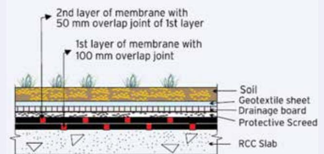
Fig. 4: A schematic diagram of a simplified roof garden component system
