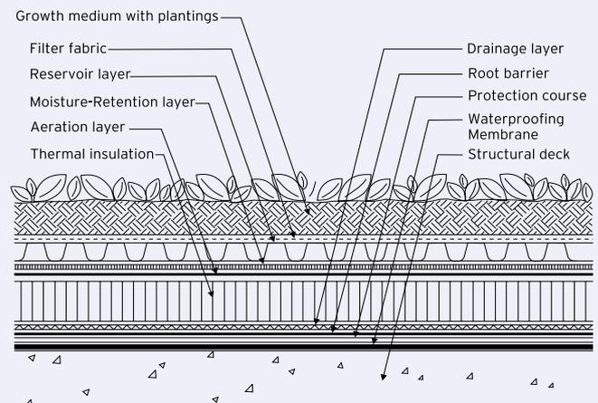
Fig. 3: A schematic diagram of an advanced roof garden component system
