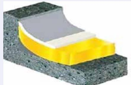
Fig. 5 : A view of PU foam insulation system over a concrete slab along with waterproofing and finishing material on top
