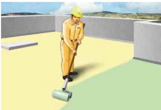
e. Application of Heavy duty acrylic based waterproofing coating over Spray applied PU Foam insulation
