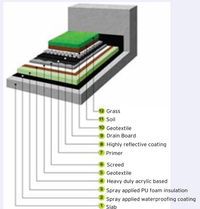
Fig. 7 : Schematic diagram for energy efficient high performance inverted roofing system for roof garden
