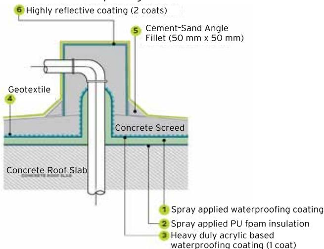
Fig. 8 : Pipe penetration detailing of a LEC system
