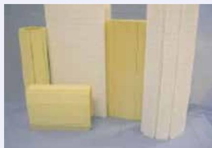
Fig. 3: View of Urethane foam insulation panels
