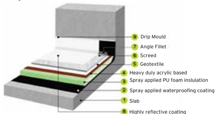
Fig. 6 : Schematic diagram for energy efficient high performance roofing system of an exposed flat roof
