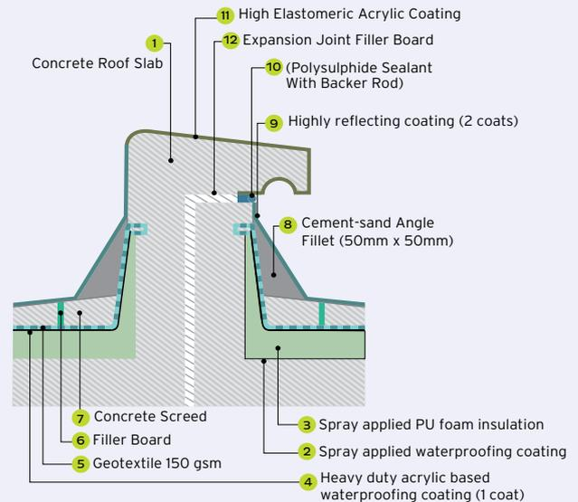
Fig. 9 : Expansion joint detailing of a LEC system
