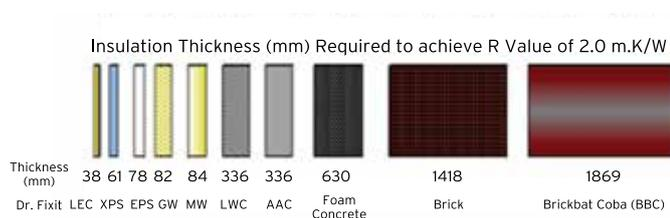
**Fig. 12 :** Comparison of thickness of different insulation material for meeting the requirement of ECBC for R value 2.1 m.C/W
