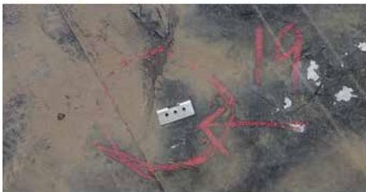
Fig. 5: Breach no 19 as detected by EFVM test
