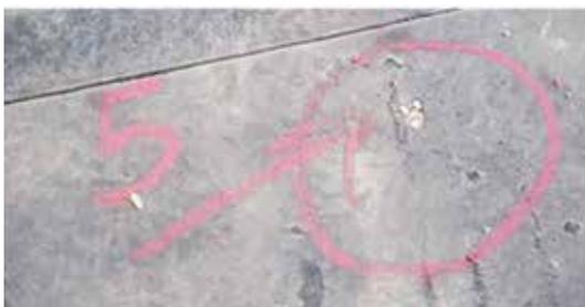
Fig. 6: Breach no 5 as detected by EFVM test
