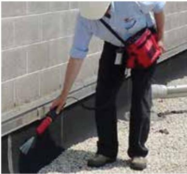
**Fig. 2:** High Voltage ELD (dry testing) is ideal for testing flashings and other vertical surfaces
