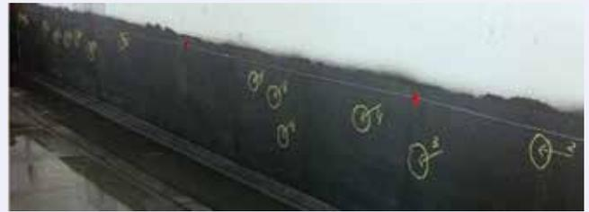
Fig. 11: Breaches identified by vector mapping test on vertical surfaces of the membrane
