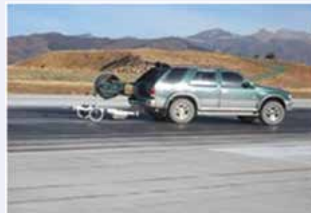
Fig. 15: GPR survey being used to evaluate the runway pavement of airport
