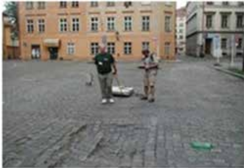
Fig. 3: GPR survey for detecting buried voids below the ground surface
