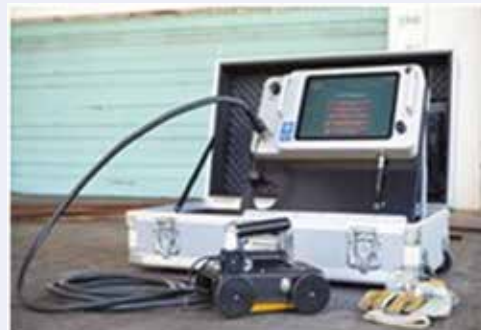
Fig. 6: GPR survey for locating post-pre- tension cables
