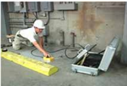
Fig. 10: GPR survey being used for measuring the depth of RCC slab
