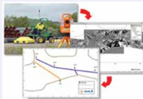
Fig. 2: GPR survey for utility mapping and their location mapping (bottom drawing) along with their 3D view of the location (top right)
