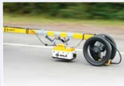
Fig. 12: GPR survey being used to evaluate the characteristics of road pavement
