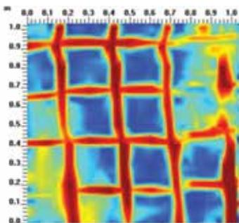
**Fig. 2c:** Cross sectional RCC profile having rebar. Data taken by 1000 MHz GPR. (Grid1x1)
