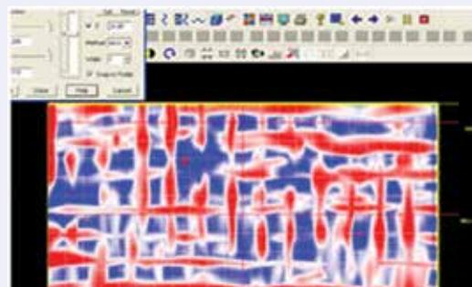
Fig. 3: C-scan - Bottom layer of rods
