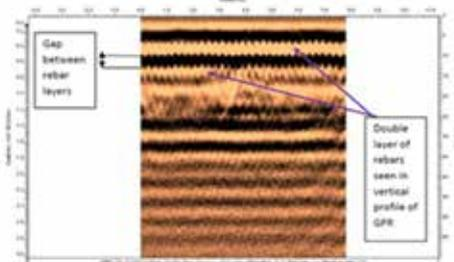
**Fig. 2a:** GPR profile of double layers of rebar. Data taken by 1000 MHz antenna based GPR
