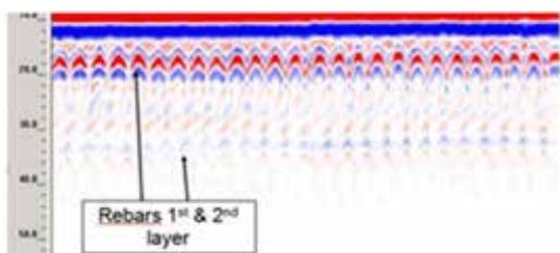
Fig. 1: Line scan for the RCC slab
