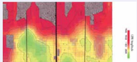
(b) GPR rebar level attenuation
