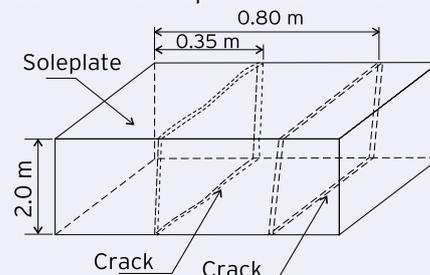
Fig. 2: 3-D representation image of the cracks
