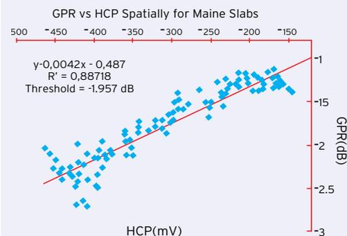
**Fig. 2:** Correlation curve between half-cell potential readings and GPR attenuation
