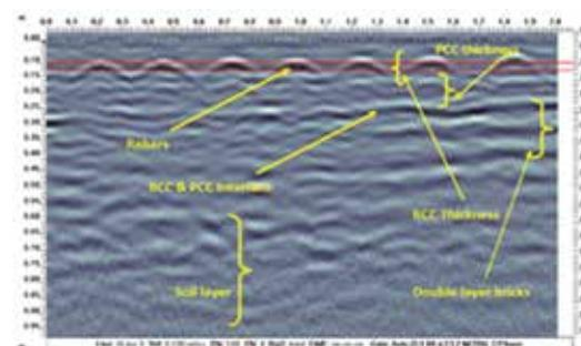
Fig. 1a: RCC pavement profile collected by 1000 MHz antenna based GPR
