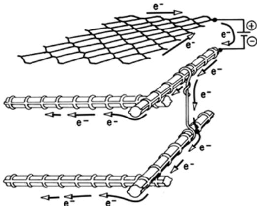
Fig.1: Schematic diagram of impressed current CP system
