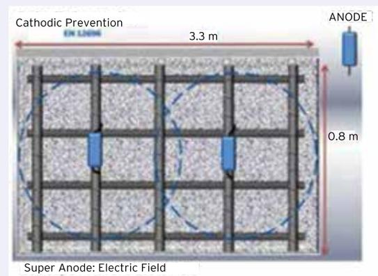
Fig. 4: Schematic diagram showing installation of Sacrificial Galvanic anode
