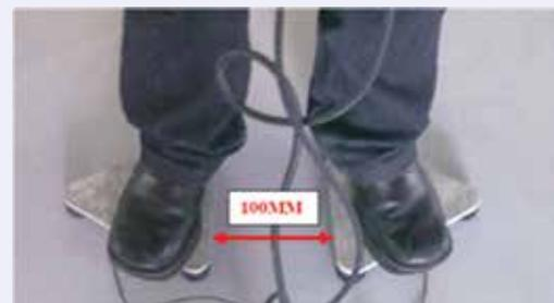
Fig. 28: Checking antistatic property of self-levelling epoxy flooring
