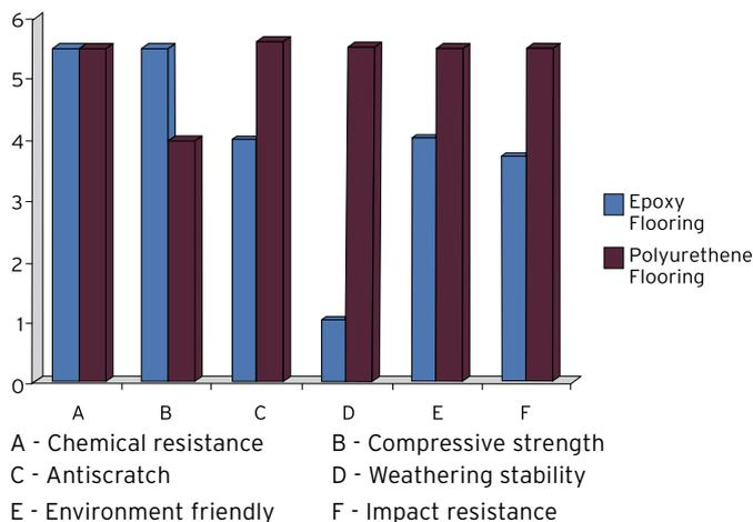
**Fig. 8:** Comparison of various properties between epoxy and polyurethane coatings
