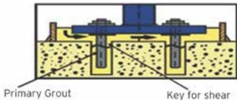
**Fig. 17:** Schematic diagram of grouting below base plate and foundation bolt pocket
