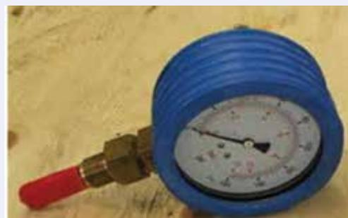
Fig. 4: Hydraulic pressure gauge
