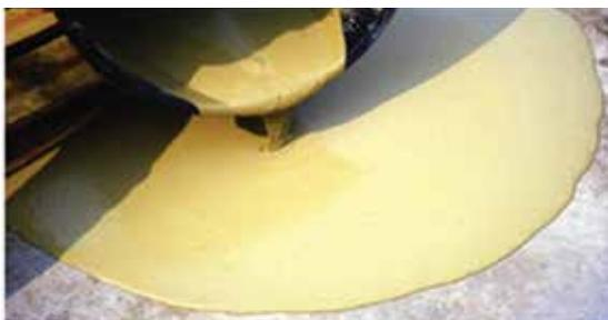
Fig. 1: View of flow of a grout material
