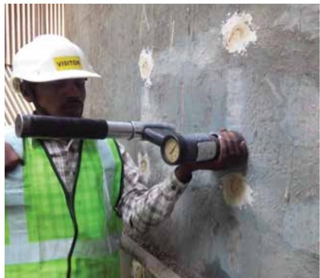
Cut and Pull out(CAPO) test for in-situ compressive strength of concrete
