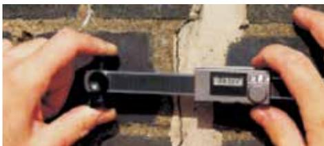
Fig. 1: Digital crack measuring gauge
