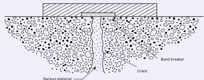
Fig. 5: Flexible sealing
