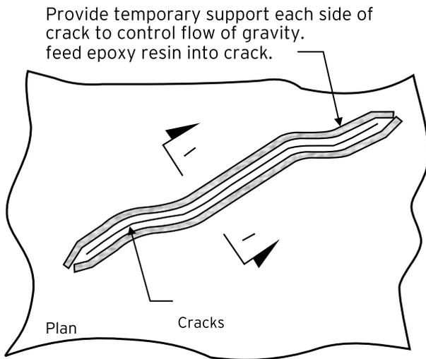
Fig. 4: Horizontal surface crack repair detail
