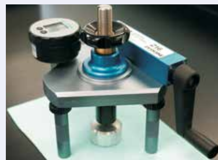
Fig. 8: Pull off test on concrete repaired surface
