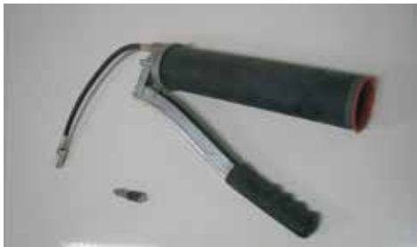
Fig. 2 a: Packer and Injection hand pump
