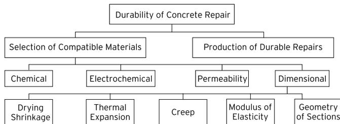
Fig. 1: Factors affecting durability of concrete repairs
